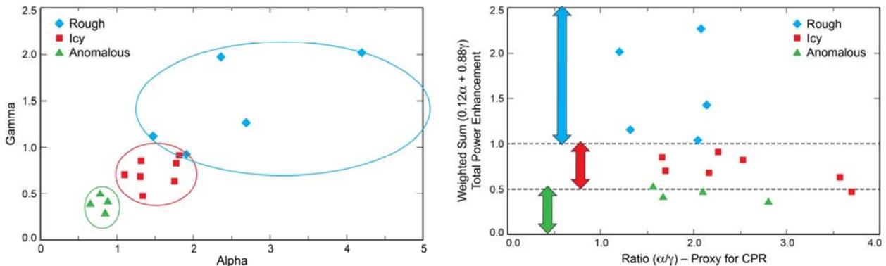
**Fig. 1.** Scatterplots of  $\alpha$  vs.  $\gamma$  (left) and of ratio ( $\alpha/\gamma$ ) vs. weighted sum [ $0.12\alpha + 0.88\gamma$ ] (right) for the 4 nonpolar craters and 12 polar craters studied using LRO Mini-RF 13-cm wavelength data. Ratio ( $\alpha/\gamma$ ) is a proxy for CPR; weighted sum is the total power enhancement. There are 3 separable crater classes: Icy, Rough, and Double-Bounce.
