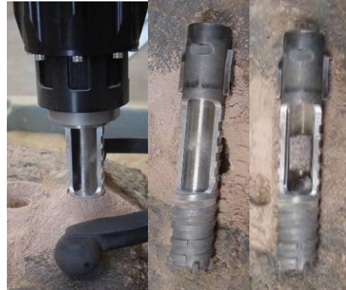
Figure 4. The Preview Bit. Left: after reaching the target depth of 2.5 cm, break-off tube is rotated to shear and capture the core. Once the tube is fully closed (Center), the core cannot fall out. To view the core, the drill is moved to a horizontal position and the inner break-off tube is rotated back to expose it. (Right)
