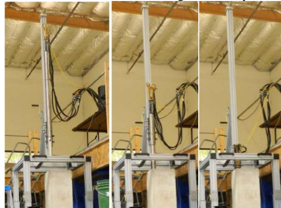
Figure 3. Drilling progress into a 2 m limestone column.
