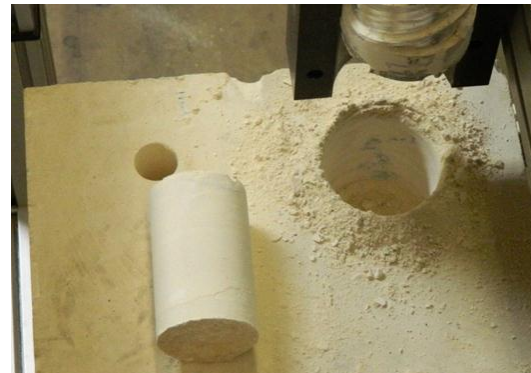
Figure 4. The recovered core samples were 57 mm diameter and 100 mm long. Core recovery was 100%.
