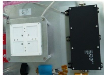
Figure 1. Engineering model of sensor unit and flight model electronics unit of BepiColombo MDM (Mercury Dust Monitor).
