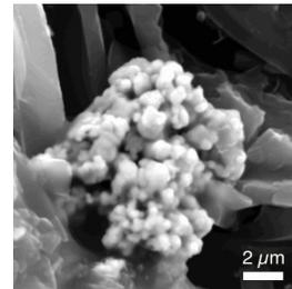
Fig. 2. SEM: Aggregate of Ag grains in the UCM matrix.
