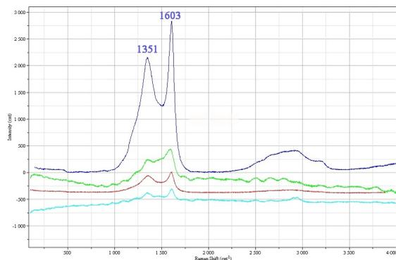
Fig.4. Raman spectra of UCM sample #2010-4.
