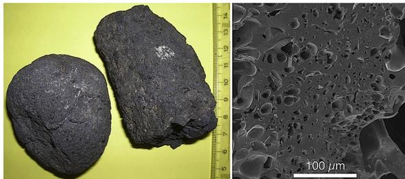
Fig. 1. Typical UCM cobbles (centimeter scale) and SEM image of the porous UCM matter
