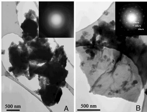
Fig. 3. TEM BF and SAED patterns of carbon particles from a UCM sample. A: amorphous. B: co-oriented mono-crystalline slightly textured  $\alpha$ - and  $\beta$ -carbynes.
