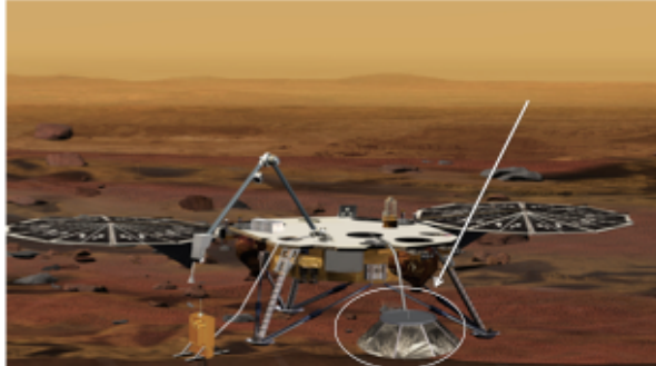
Figure 1: SEIS deployed on the ground next to the the INSIGHT Lander
