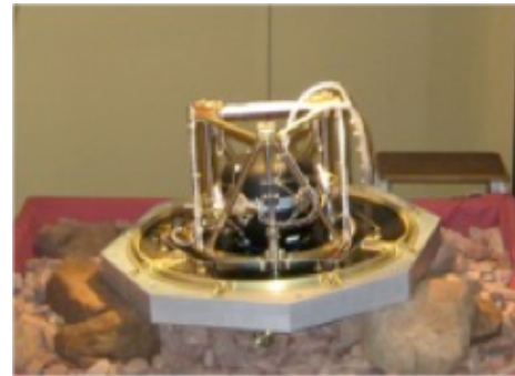
Figure 2: SEIS breadboard (courtesy MPS)
