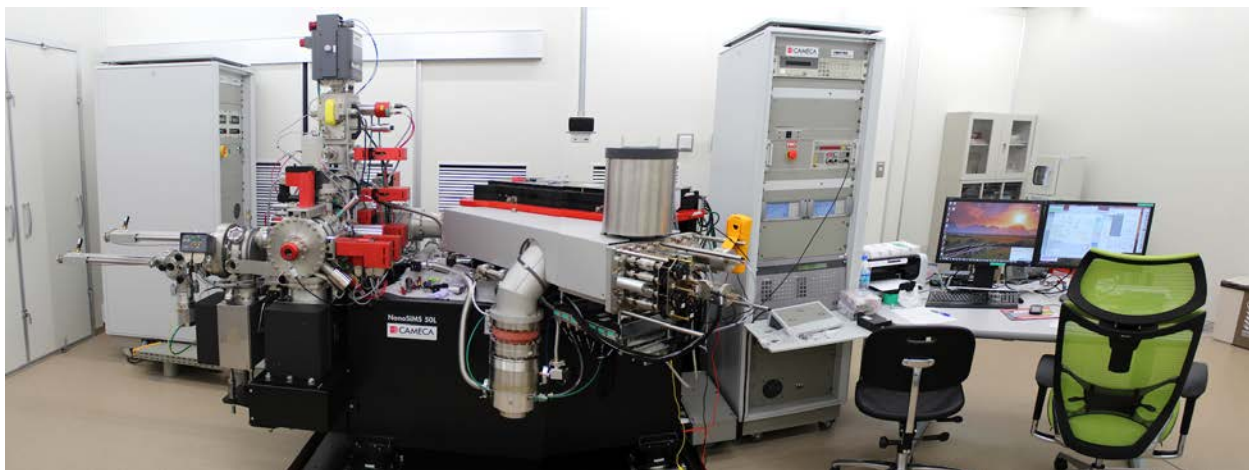
Figure 1. The JAMSTEC NanoSIMS 50L in a clean room (Class 10,000)
