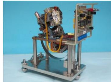
**Figure 3 :** Last 1 axis-VBB prototype (VBB-41) with its proximity electronic
