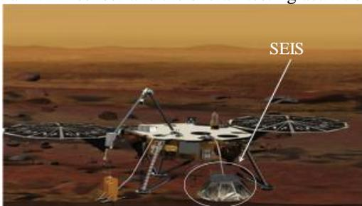
**Figure 1 :** SEIS deployed on the ground next to the the InSight Lander
