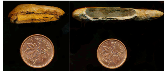
Figure 1: Cross section of nodules from Devon Island. Image on left shows a more oxidized nodule. Image on right is primarily pyrite and with a gypsum coating. Penny for scale.
