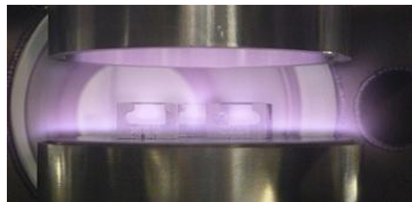
Figure 2. GEC Reference Cell used in this study. Three samples employing different layers were exposed to an argon plasma. High pressure/ high power conditions (as described in Table 1) were employed for a maximum of 15 min.
