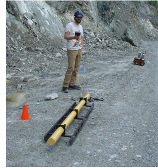
Figure 1. EMIS data being recorded 10 m behind the test rover during June 2011 deployment.
