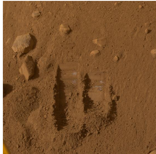
Figure 1. Dodo-Goldilocks trench, sol 14 showing exposed water-ice table. Excavated by Phoenix's Robotic Arm.
