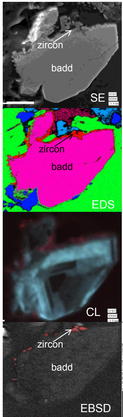
Figure 1: SE image of euhedral microbaddeleyite (badd). Note microgranular texture. Scale bar = 5 microns; EDS phase map showing baddeleyite, zircon rim and host plagioclase/ maskelynite (green); CL image revealing planar sector zoning typical of igneous crystallization plus zircon rim (magenta); EBSD band contrast map indicating that all phases are now amorphized due to shock except for zircon rim crystallites.
