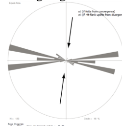
Figure 4. Stress analysis of mountain ridges at 200 W: stress arrows are (1) \sigma_1 if folds are formed from convergence or (2) \sigma_3 if rift-flank uplifts from divergence
