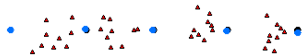
Figure 4. Rover sites along the traverse (blue dots) and the features or tie points (red triangles). The black dots represent rover reference positions measured using standard GPS, while the overlaid blue dots represent the same rover positions as calculated by the BA. The measurement error of rover position is within 4 cm due to GPS placement.
