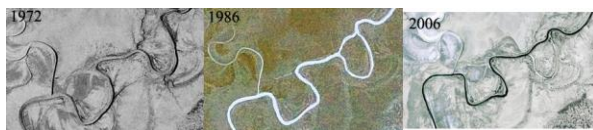
Fig. 1. Evolution of meandering channel found within the target site. One can see that meander loop was cutoff around 1986. By 2006, the loop that was cutoff has been completely abandoned. (Images obtained from Google Earth and USGS Earth Explorer)
