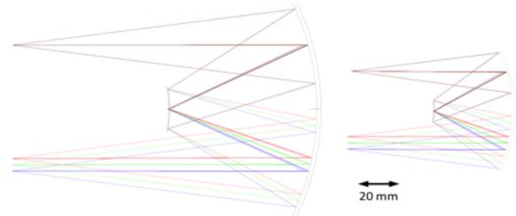
**Figure 3. Optical ray traces for the M3 (left) and UCIS (right) imaging Spectrometers.**
