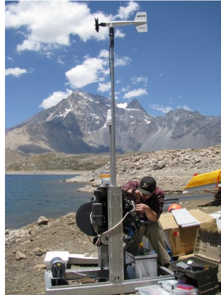
Figure 1: Installing the Lake Lander meteorological station.
