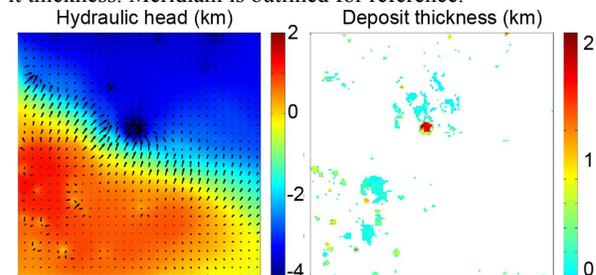
**Figure 3.** Snapshot of the hydraulic head and flow vectors at Gale Crater (left) showing a convergence of flow into the deep hydraulic sink at the crater, and the predicted deposit thickness (right).
