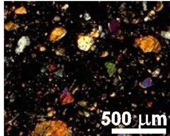
Figure 2: polarizing optical microscopes image of a thin section of NWA 6687. Yellow to blue crystals are olivine; white crystals are plagioclase; black areas are glass; transmitted light, crossed polars.
