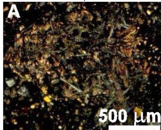
Figure 3: blow-up image of the inclusion A in Figure 1; elongated grey crystals are plagioclase, cream yellow crystals are pyroxene, black areas are glass; transmitted light, crossed polars.
