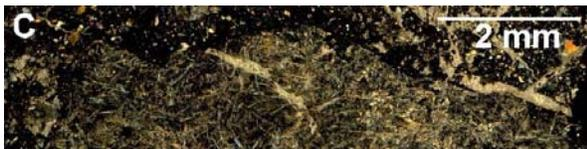
Figure 5: blow-up image of the inclusion C in Figure 1; elongated grey crystals are plagioclase, cream yellow crystals are pyroxene, black areas are glass; transmitted light, crossed polars.
