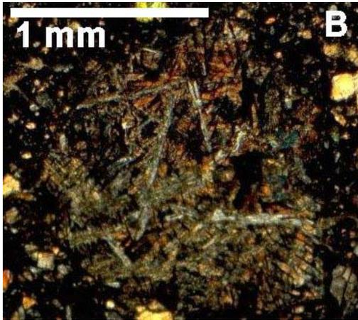
Figure 4: blow-up image of the inclusion B in Figure 1; elongated grey crystals are plagioclase, cream yellow crystals are pyroxene, black areas are glass; transmitted light, crossed polars.
