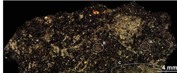
Figure 1: photomosaic of polarizing optical microscopes images of a thin section of NWA 6687. Yellow to blue crystals are olivine; black areas is matrix; A, B and C are medium-grained basaltic inclusions; transmitted light, crossed polars.
