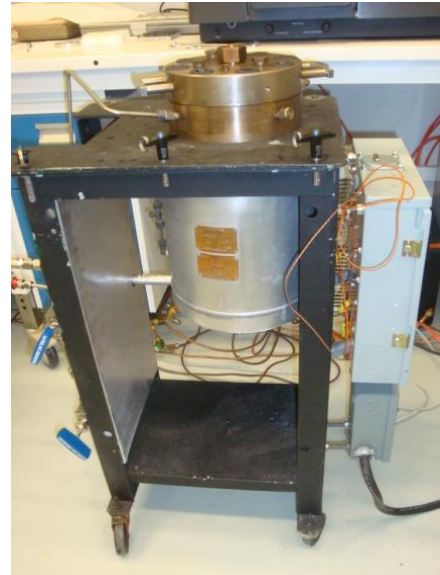
Figure 1: The Venus simulation chamber at NASA Goddard.
