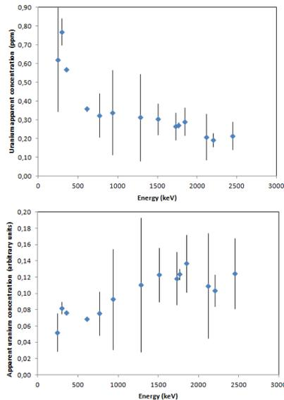
Fig. 2: Apparent uranium concentrations as a function of energy for two scenarios: Top: assuming all uranium decay products are in the soil; Bottom: assuming they are in the atmosphere.
