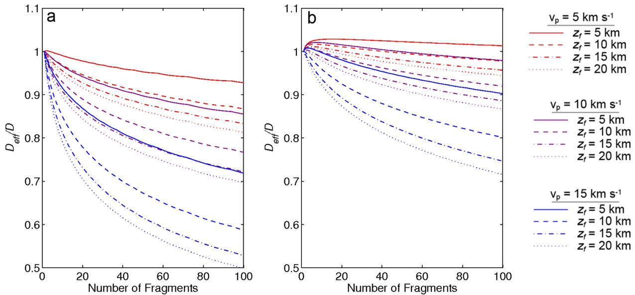
Figure 2: The ratio of  $D_{eff}/D$  versus  $N$  for initial projectile diameters (a) 50 cm, and (b) 1 m.
