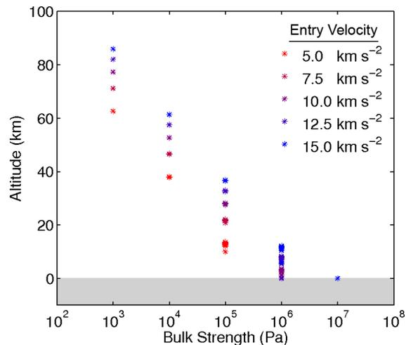
Figure 1: Fragmentation altitude,  $z_f$ , versus bulk meteoroid strength in the martian atmosphere. Color indicates initial projectile velocity. Diameter and entry angle only influence  $z_f$  for projectiles penetrating deep into the atmosphere.
