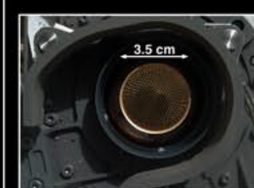
CheMin sample inlet as viewed by MAHLI on Sol 34. This is a focus merge product.
