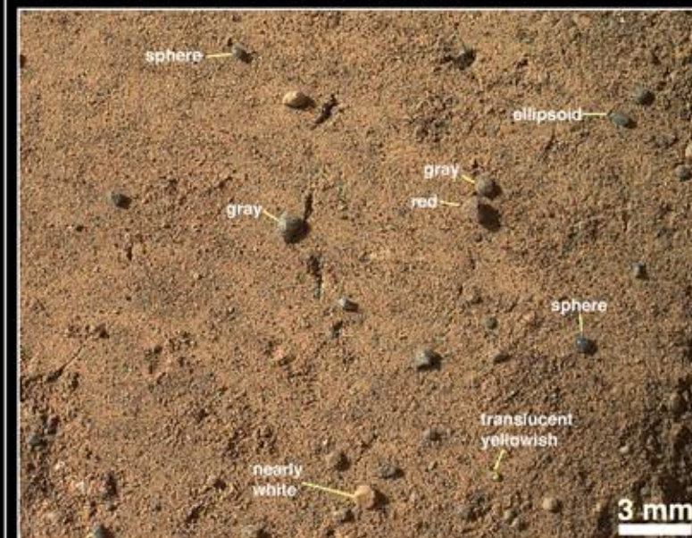
Portion of a Sol 58 image of Rocknest Sand Shadow sediment flattened by the rover's front left wheel. Larger grains (mm-sized) exhibit a variety of colors and shapes. Finer grains are < 150 \mu\text{m} in size, perfect for passing through Curiosity's sample handling system and sieves for delivery to the CheMin mineralogy instrument.
