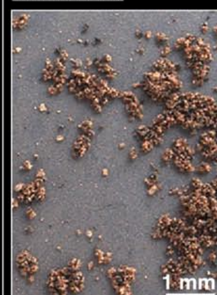
This is a portion of grains sieved to \leq 150 \mu\text{m} size from the 5th Scoop at the Rocknest Sand Shadow. APXS observed this sample and CheMin and SAM received portions from the same sample. This is a sub-frame of a larger MAHLI image acquired on Sol 95 at 21.2 \mu\text{m}/\text{pixel} .
