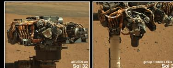
MAHLI camera head inspections, dust cover closed, prior to first-time opening on Mars. Goal was to ensure debris raised during terminal descent would not obstruct dust cover motion.
