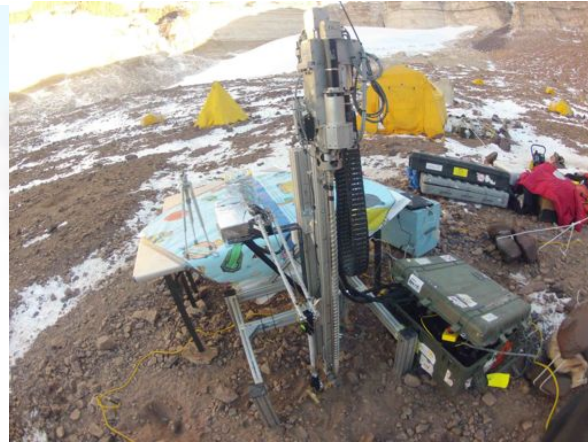
Icebreaker rotary-percussive drill was tested with integrated sample transfer arm and instrument mockups, commanded remotely (with time lags inserted) end-to-end from NASA Ames to the University Valley site in January 2013.
