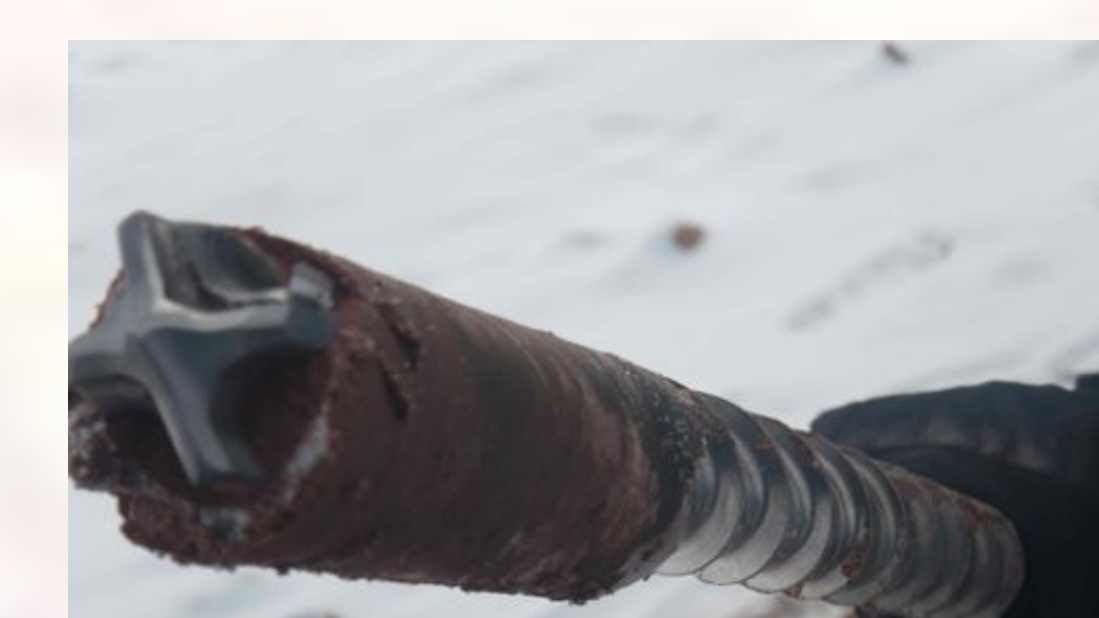
Thawing and refreezing of cuttings led in Antarctic tests to choking faults.
