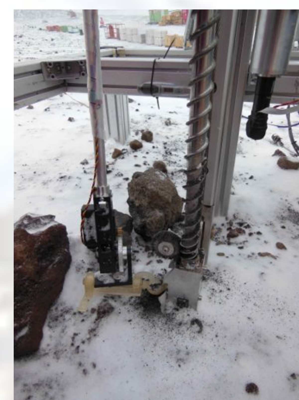
A brush removes captured cuttings into a sample-transfer scoop. Air gap breaks contact chain for planetary protection.
