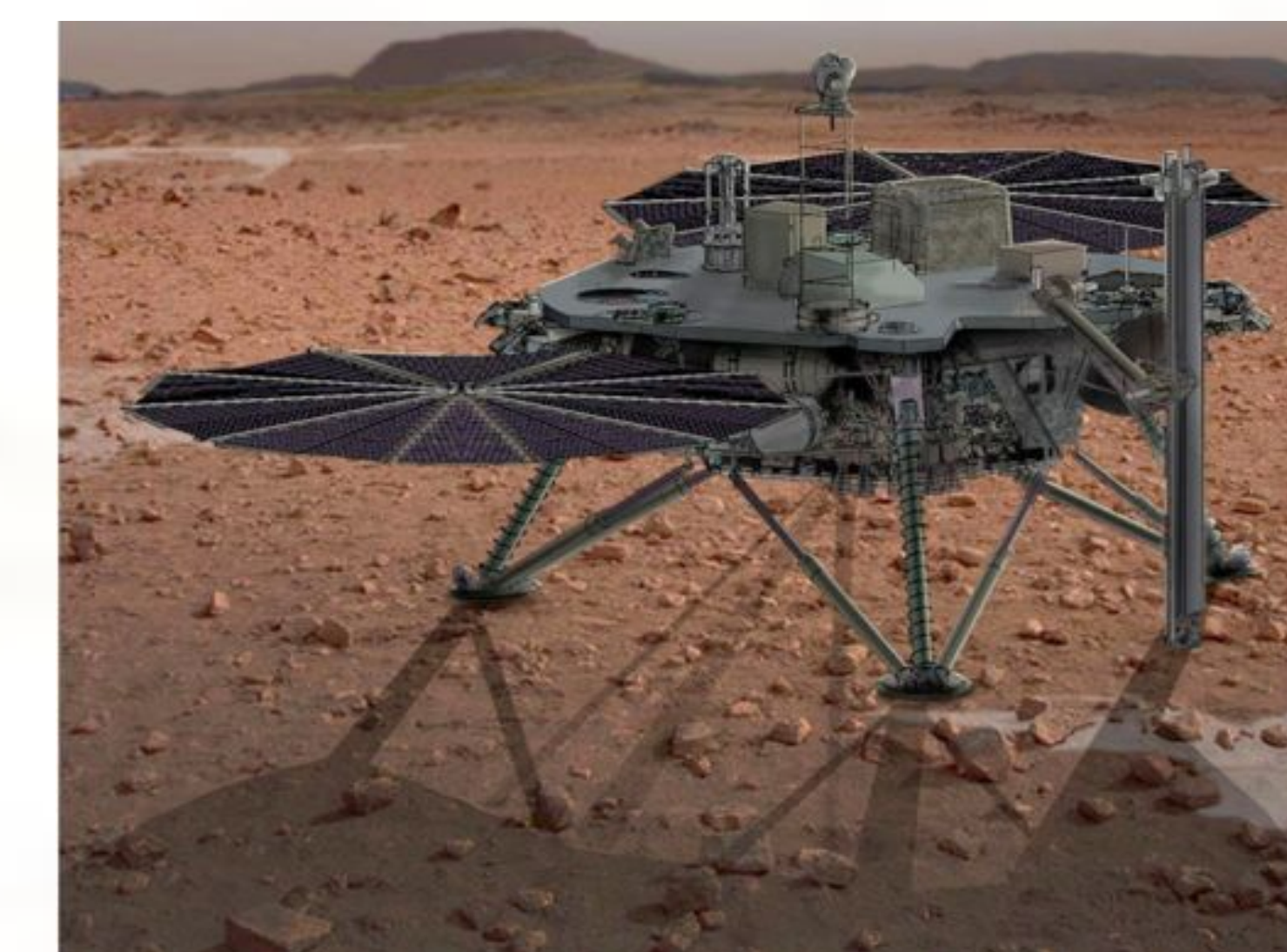
Icebreaker drill and life-detection science payload on a Phoenix-based platform [LM]
