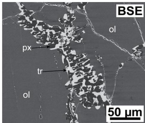
Fig. 1. BSE image of the symplectitic intergrowth texture that occurs along olivine grain boundaries in the MIL ungrouped achondrites.
