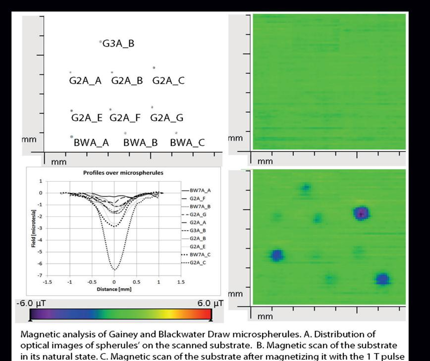
field directed into the page. D. Magnetic profiles of each spherule in horizontal direction.
