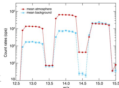
**Fig. 2:** SAM/QMS spectrum at 0.1-Da resolution, acquired on Sol 77 of the MSL mission. Background and atmosphere spectra are averages of many scans, and statistical uncertainties in these averages are plotted as error bars.
