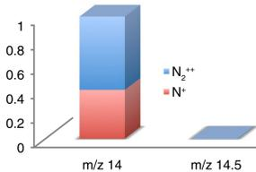
**Fig. 1:** Nitrogen ions contributing to m/z 14 and 14.5. The objective is to determine the  $^{14}\text{N}/^{15}\text{N}$  isotopic ratio from the data. If the fraction of the signal at m/z 14 from  $\text{N}^+$  is known, then the ratio of the remaining signal at m/z 14 to the signal at m/z 14.5 gives the isotopic ratio.
