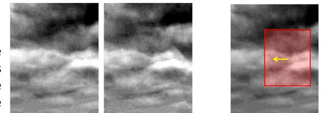
**Far Right:** The centre portion of the second (right-hand) frame is overlain in red on the earlier frame at the position of best correlation. The vector which returns it to the centre represents the wind direction.
