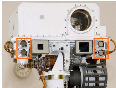
**Above:** Orange boxes indicate the NavCam imagers on the rover's remote sensing mast
