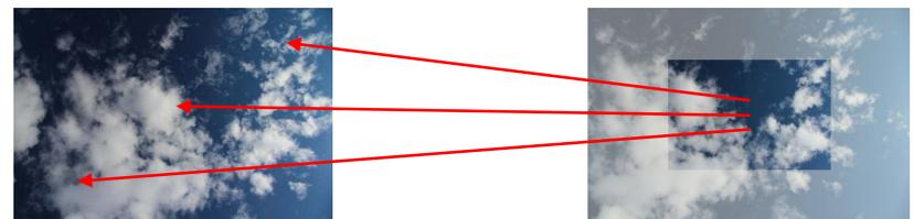
**Above:** In the cross-correlation technique, the centre portion of one image is compared to all regions of an earlier image in the sequence to find the area of greatest similarity. The vector between that location and the centre represents the wind direction, here almost directly leftward in images from the Canadian Arctic. The technique has shown success with images from both Earth and Mars, with a variety of cloud morphologies.
