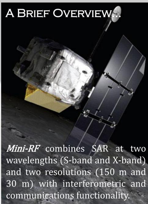
Mini-RF combines SAR at two wavelengths (S-band and X-band) and two resolutions (150 m and 30 m) with interferometric and communications functionality.
