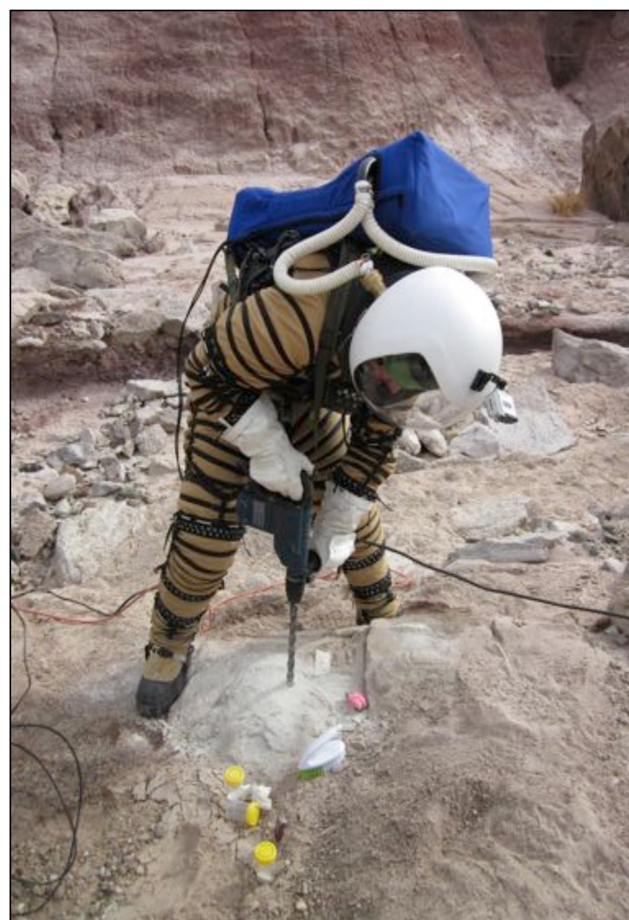
Figure 1: Rotary Percussive drilling in suit. Note cuttings around the hole.
