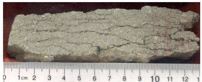
Figure 1. Example of “decompression cracks” on a cut surface of a Lonar Class 2 shocked altered basalt. Note red hematite to right and greenish tint of alteration minerals throughout.
