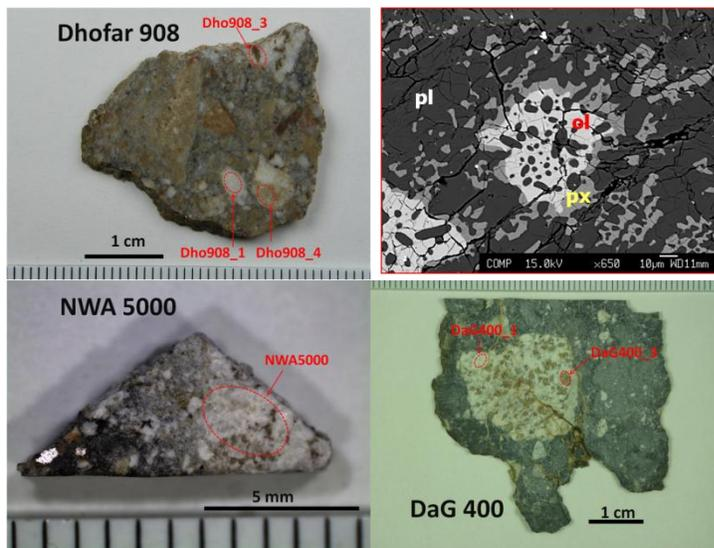
Fig. 1. Photomicrographs of the three feldspathic lunar meteorites with troctolite clasts. Red circles indicate measured spots (about  $3 \times 2$  mm in size) for reflectance spectral analyses.
