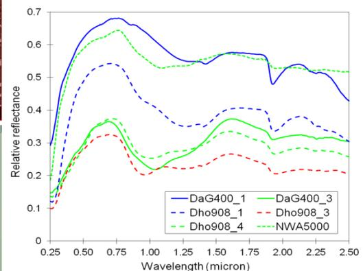
Fig. 3. Reflectance spectra of troctolites in the three samples. Blue spectra is plagioclase dominated, green ones are olivine dominated, and a red one is low-Ca pyroxene dominated, in the reflectance spectral viewpoint.
