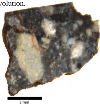
Figure 1. Scanned thick section of feldspathic regolith breccia lunar meteorite Dar al Gani (DaG) 400 [3]. Many small rock fragments (clasts) of impact melt breccias, anorthositic lithologies and mineral fragments are consolidated together in a fine grained glassy matrix.
