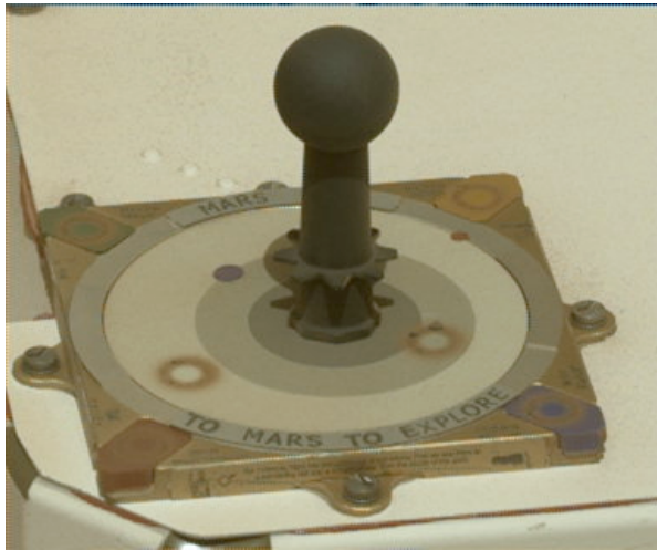
Figure 2: The Mastcam caltarget imaged on sol 72 of Curiosity's mission through the Mastcams L0 filter. The caltarget base is a square 8 cm on a side. Image ID: 0072ML055600000E1. Image credit: NASA/JPL-Caltech/Malin Space Science Systems
