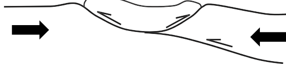
Fig. 6. Sketch cross-section, not to scale, of compressional tectonics acting on a part-filled impact basin.
