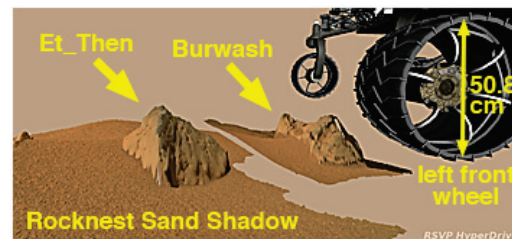
Fig. 2. Example of engineering activities that used the MAHLI; this is a terrain visualization product created from MAHLI stereo pair images of rocks Et_Then and Burwash. The data were obtained and processed to assist with robotic arm positioning of MAHLI and APXS and to explore techniques for future MAHLI assistance with placement of Curiosity's robotic arm tools and instruments.
