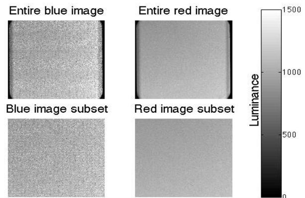
A central 800 x 1000 pixel subframe of each image is used to exclude the dark-pixel areas of the images. The mean luminance is found for the blue image (1034 +/- 61) and for the red image (1008 +/- 130). The ratio of these mean values provides the blue to red ratio for the observation: B/R = 1.0252 +/- 0.1434. B/R ratios equal to within 0.5% of these values were obtained using the linearized product versions of the same images.
