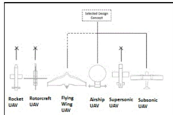
**Final Concept.** The finally vehicle was designed to have 70% of the neutral buoyancy at cruise altitude from the helium lifting gas, and the remaining lift force from the flow over the airfoil section. In keeping with the endurance, power and cruise velocity requirements, the powerplant was designed as a solar powered electric propeller, and was designed to operate continuously at a low velocity.
