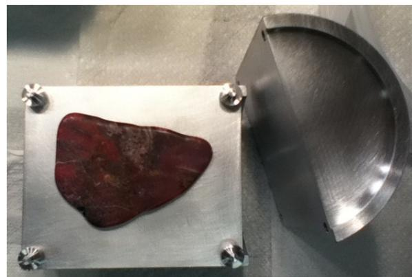
**Fig. 3** Thin-slice insert with the halves separated. A sample (in this case, terrestrial rhodonite) lies flat on the face of the bottom half. Separators are visible at each corner of the face.
