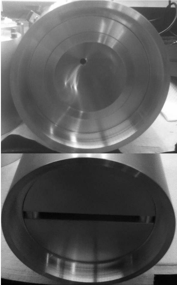
**Fig. 2** Inserts placed in the primary chamber, with lid removed. (Top) Nested sleeves. (Bottom) Thin-slice insert.
