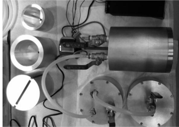
**Fig. 1** Top view of the pycnometer. The primary chamber is upper right. Secondary chambers are bottom right. At left are the inserts for the primary chamber.
