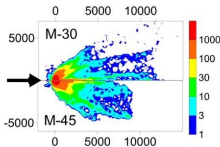
**Fig. 3.** Number of microtektites per  $1 \text{ cm}^2$  as a function of a distance (in km) from the impact point (0,0). Only half of the “map” for each variant is depicted. A black arrow shows the impact direction. M-30: a 1-km-diameter asteroid striking at a  $30^\circ$  to horizon into a 300-m-deep water layer; M-45: same projectile size, but the impact angle is  $45^\circ$ .
