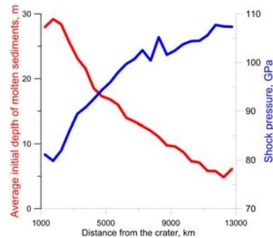
**Fig. 5.** Initial depth of molten material (red line and left axis) its and maximum shock compression (blue line and right axis) as a function of distance from the parent crater.
