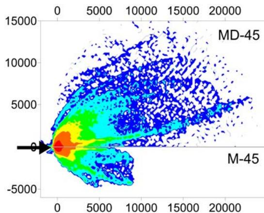
**Fig. 4.** Comparison of a  $45^\circ$  impact into a 300-m-deep water layer (M-45) and into a dry surface (MD-45). All colors are the same as in Fig.3.
