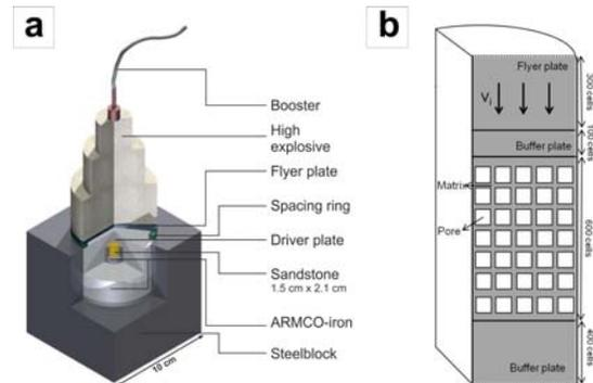
Fig. 1. (a) Experimental set-up for the shock recovery experiments. (b) Illustration of the meso-scale model set-up including the sample with a defined number of well resolved pores.
