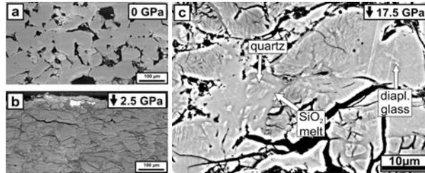
Fig. 2. Comparison of quartz in SEM-BSE images of (a) unshocked and (b) shocked (2.5 GPa) Seeberger sandstone. Note the total closure of pore space. (c) Formation of diaplectic quartz glass and SiO<sub>2</sub> melt (homogeneous zones without fractures) in the sandstone shocked to 17.5 GPa.
