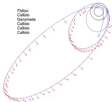
Figure 3. Example trajectory to set up Callisto capture.
