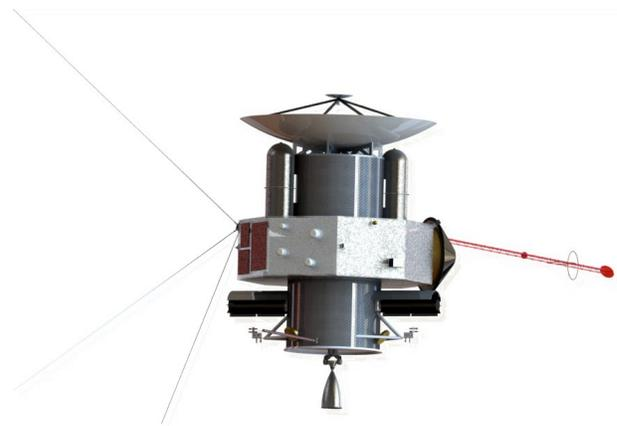
**FIG. 4:** Design of the main spacecraft, including the probe, 4 ASRGs, a 3.5 m high gain antenna, the main thruster.
