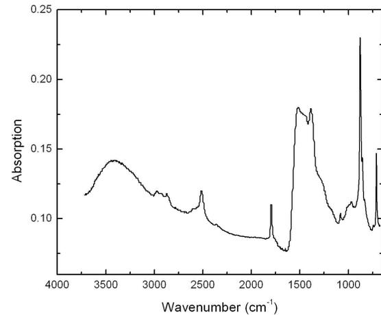
**Figure 3.** Average IR spectra obtained by combining the 182 individual mosaic spectra of a  $\sim 150\text{ }\mu\text{m}$  grain from SM12 that largely consists of carbonates.
