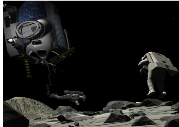
Figure 1. Screenshot of MMSEV NEA simulation showing MMSEV with one EVA crewmember attached to an astronaut positioning system (APS) and a second free-flying using an EVA jetpack.
