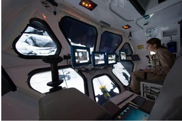
Figure 3. Test subject inside the Gen 2A MMSEV. Video walls displaying the NEA simulation can be seen through the windows.
