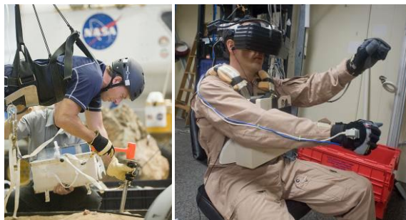
Figure 4. Test subject performing exploration EVA tasks in simulated microgravity using ARGOS (left) and the VR laboratory (right).
