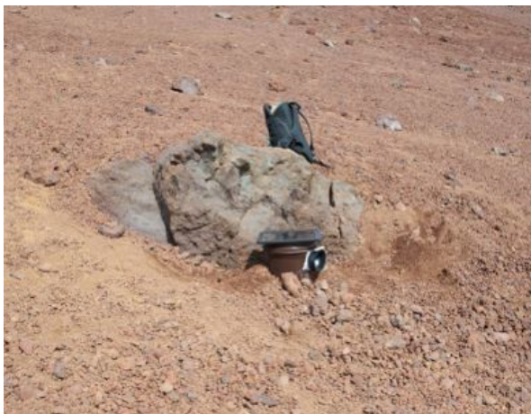
Figure 1. Time-lapse infrared camera in the field. The camera looks to the right (south).
