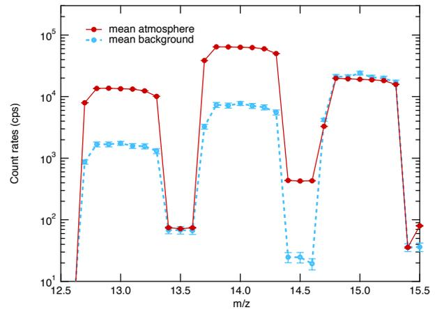
**Figure 1:** SAM/QMS spectrum at 0.1-Da resolution, acquired on Sol 77 of the MSL mission. Background and atmosphere spectra are averages of many scans, and statistical uncertainties plotted as error bars.
