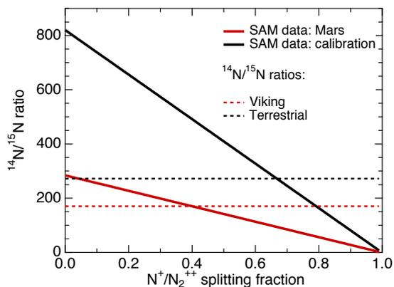
**Figure 3:** Nitrogen isotopic ratio as a function of the  $\text{N}^+/\text{N}_2^{++}$  splitting pattern (an intrinsic characteristic of the SAM/QMS). With terrestrial  $^{14}\text{N}/^{15}\text{N}$  in the calibration gas, the splitting fraction lies at the intersection of the black lines. A planned measurement of the calibration gas isotopic ratio will derive the splitting fraction determining  $^{14}\text{N}/^{15}\text{N}$  on Mars from the solid red line.
