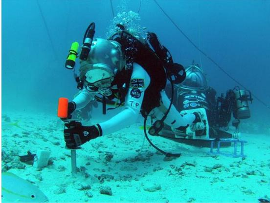
Figure 4. EVA crewmember hammering geophysical array anchor while attached to a foot restraint on the Deep Worker submersible (MMSEV analog). Photo credit: NASA/M.Widick.
