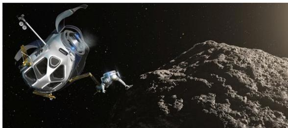
Figure 2. Depiction of an MMSEV with a crewmember performing extravehicular activity (EVA) in a foot restraint on an astronaut positioning system (APS) near a NEA. Image credit: NASA.
