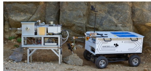
Figure 3: Second generation portable LDRIMS during preliminary field testing with rover [6].
